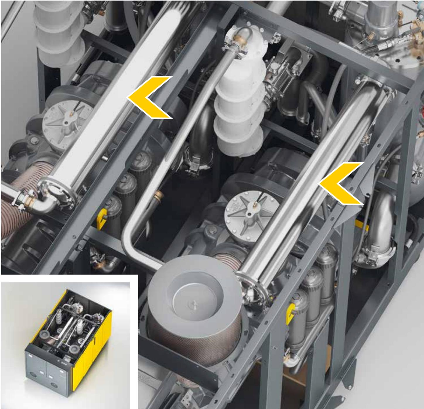
In comparison to plate heat exchangers of adequate cooling capacity, shell and tube heat exchangers made from copper-nickel alloy (CuNi10Fe) are less susceptible to contamination than plate heat exchangers. They are also more robust and the lines and exchangeable inserts can be cleaned very easily. In addition they are seawater-proof, which means that they are suitable for compressors used in shipping operations and operate with minimal pressure loss.
