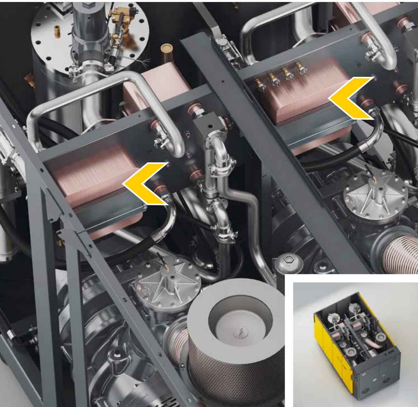
Two copper plate-soldered stainless-steel plate-type heat exchangers assure excellent heat transmission thanks to high cooling capacity plate corrugation design – the perfect choice for applications with clean compressor cooling water.
